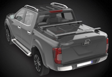
Cross bars mount easily into the 'C' channel
